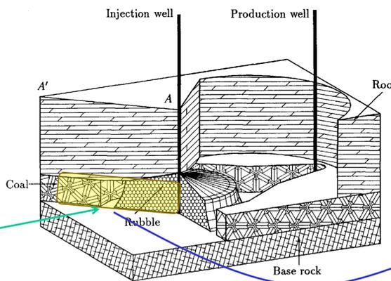
A 3-D representation of UCG with partial roof collapse [1]
