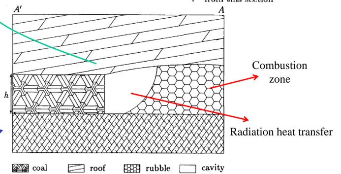
A simplified model of partial roof collapse scenario in UCG process; The overall process is mass-transfer limited [1]
